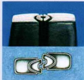
With applicator jaws properly aligned (above) and misaligned (below).
